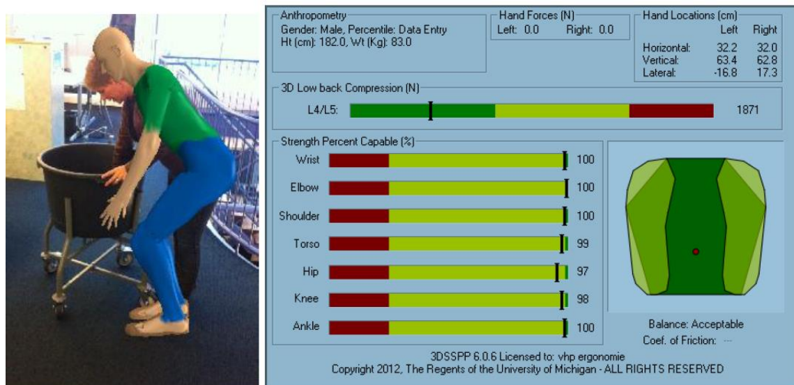
Figure 2. 3DSSPP-model analysing working with the Tub holder. Back load is 1871 N, this is without lifting.
