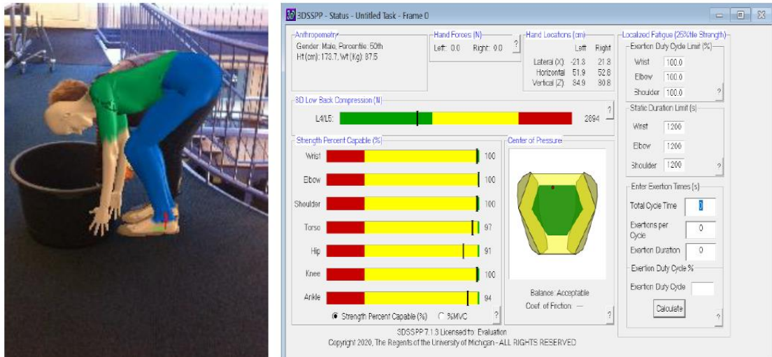
Figure 1 Analysing the traditional way of working with 3DSSPP. Back load is 2894 N, this is without lifting.
