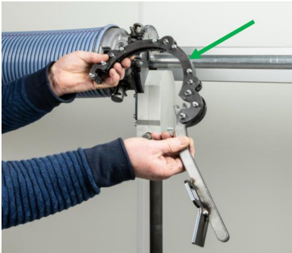
4. Lever/handle can only be closed after correct installation.
