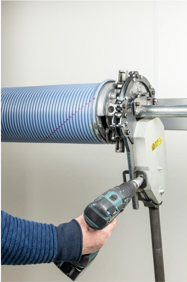
Figure 2 Application of the Industrial Torqtool using a drill: the spring is tensioned by the drill bit drive and not by manual force.
